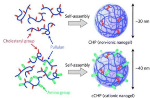
Figure 3. Schematic representation of the hybrid nanogels, adapted from 2 .
