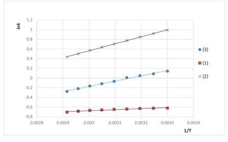
Figure 4. Graph of dependence lnk on T<sup>-1</sup> for compounds 1-3.
